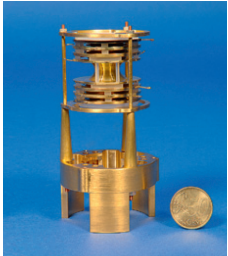
In a Penning trap single, isolated ions are observed to the highest precision.
